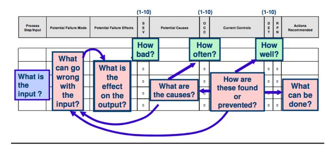
**Example:** Completing an FMEA (Failure Mode and Effects Analysis)<sup>10</sup>
