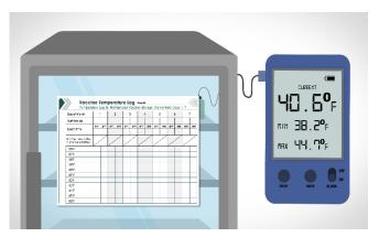
**Alt text:** A pharmaceutical-grade storage unit and digital data logger. A vaccine temperature log sheet is taped on the door of the pharmaceutical grade storage unit.
